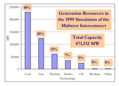
Figure 4 Generation Resources in the 1999 Simulation of the Midwest Interconnect
