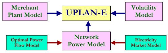
Figure A.2 Schematic of UPLAN-E
