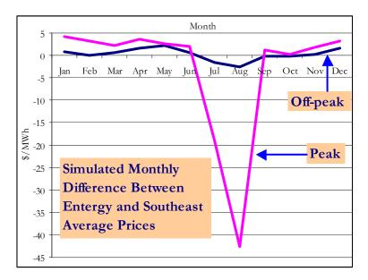
Figure 6 Simulated Monthly Differences Between the Entergy Area and Southeast Average Peak and Off-peak Prices
